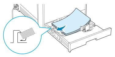
Make sure that all four corners are flat in the tray and under the corner brackets, as shown below.
